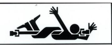
Never use your hands to clear if clogged. Never allow anyone to reach into the rotor housing. The rotor can crush and/or dismember. Keep everyone clear of the rotor until the prime mover engine is off and the hydraulic pressure has been relieved.
